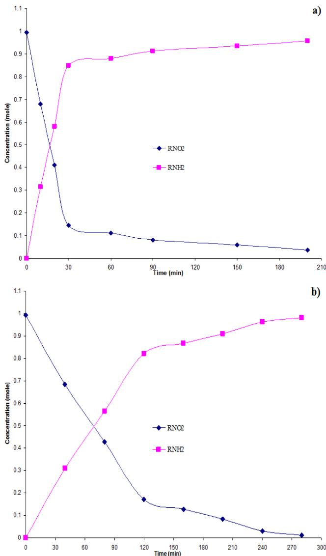
Figure 5: Dimethyl-nitrobenzene and dimethyl-aniline concentrations in solution verses time of reaction- (a) Pd/C (b) Ni
