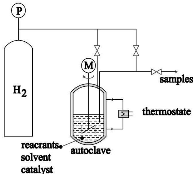
Figure 1: Experimental set-up for the liquid hydrogenation of dimethyl-nitrobenzene
