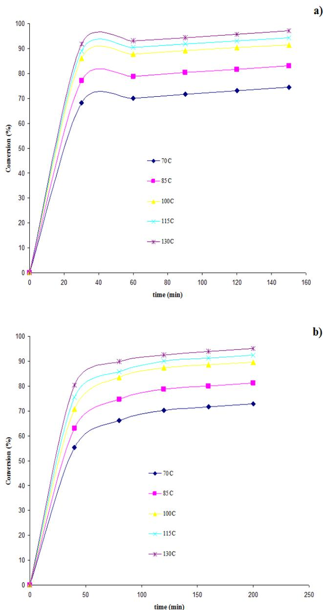
Figure 3: Evolution of the conversion level with time at different temperature- (a) Pd/C, (b) Ni
