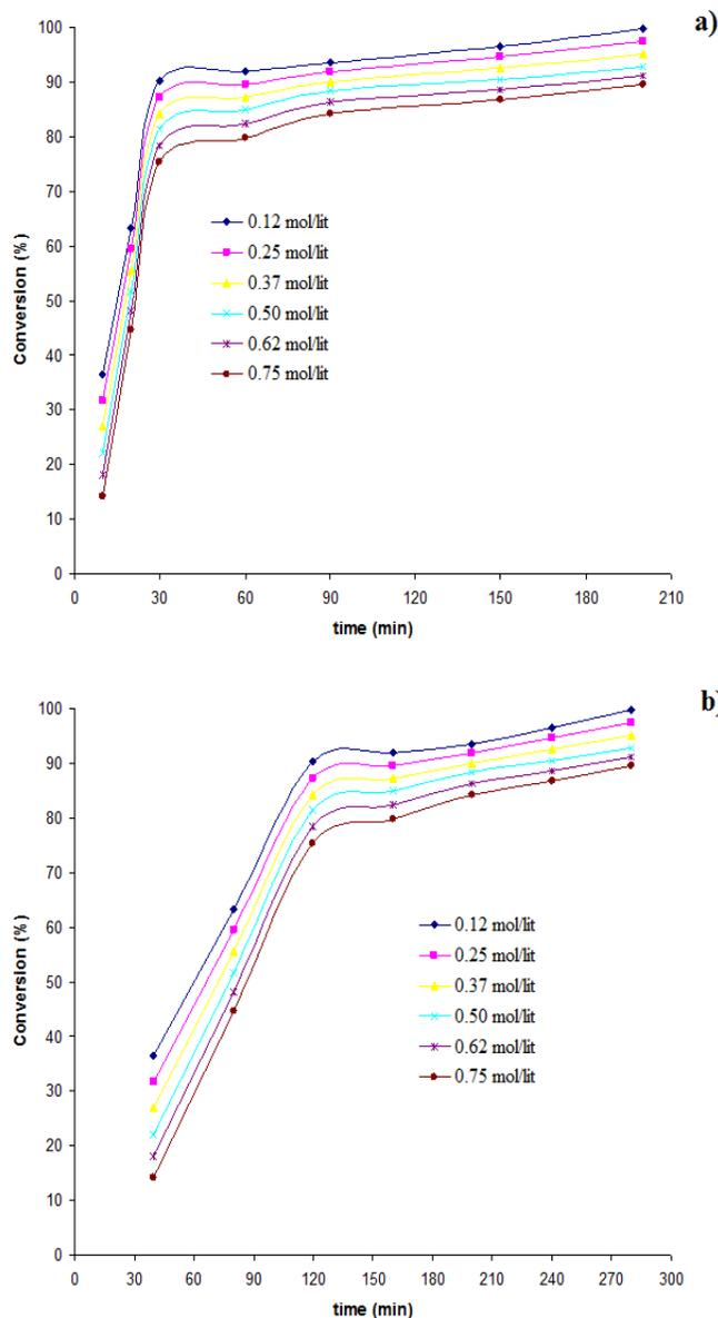
Figure 4: Evolution of the conversion level with time at different dimethyl-nitrobenzene concentration- (a) Pd/C, (b) Ni
